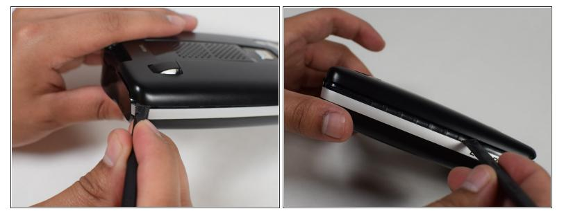
Slide the spudger around the perimeter of the radar housing until the case separates.
