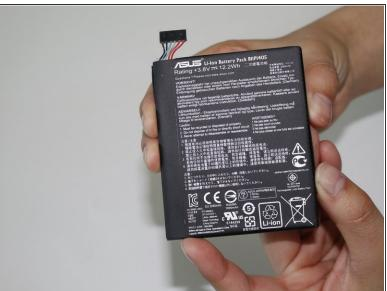
Remove the battery from the device.
