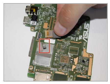
(i) Make sure you leave the tape attached to the motherboard as you will need it to fix the new camera.
