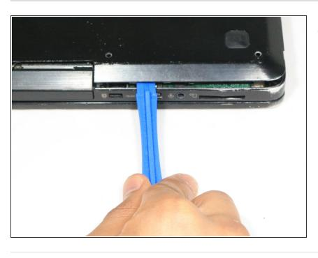
Use the plastic opening tool to pry the back panel off the base of the laptop.
