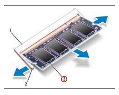
Remove the memory module from the memory-module connector.
