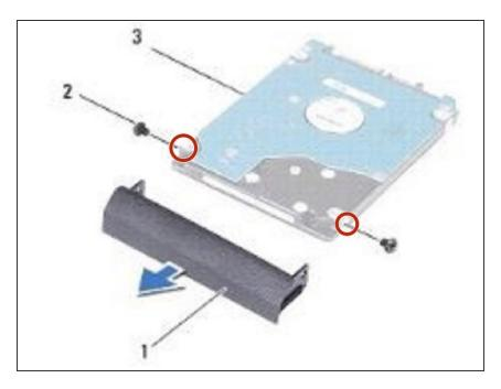
Align the screw holes on the harddrive bezel with the screw holes on the **NEW** hard drive and replace the two screws.
