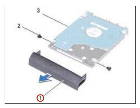
• Pull the hard-drive bezel away from the hard drive.
