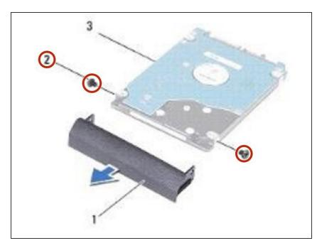
Remove the two screws that secure the hard-drive bezel to the hard drive.
