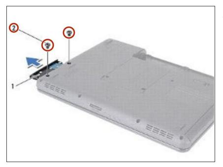
Replace the two screws that secure the hard-drive assembly to the computer base.
