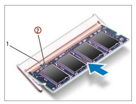
Align the notch in the **NEW** memory module with the tab in the memorymodule connector.
