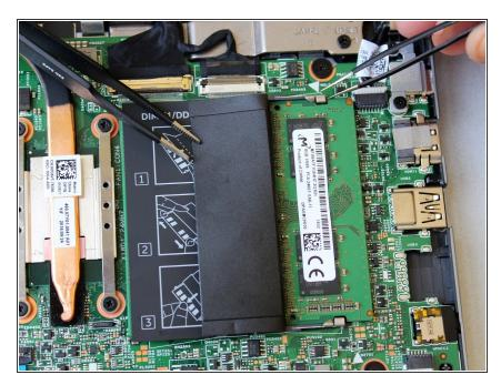
• Fold protective flaps to the side on the RAM module located in the upper right corner of the laptop.
