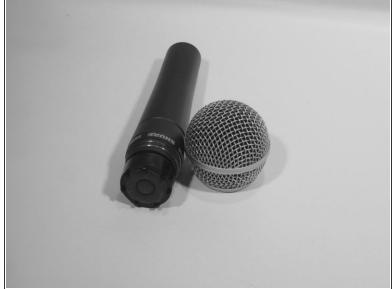
• Completely unscrew the grille and slide it off of the top of the microphone. The unprotected microphone is delicate, so place it somewhere safe while you follow the next steps.
