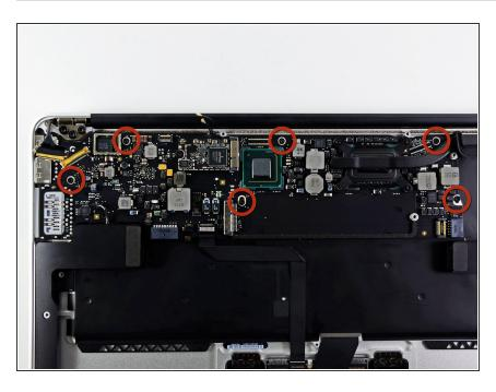
Remove the six 6.3 mm T5 Torx screws securing the logic board to the upper case.
