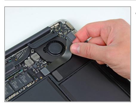
Carefully peel the I/O board cable from the top of the fan.
