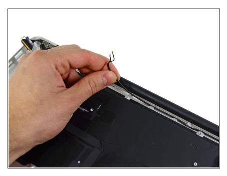
Gently de-route the antenna cables out of the channel cut into the upper case.
