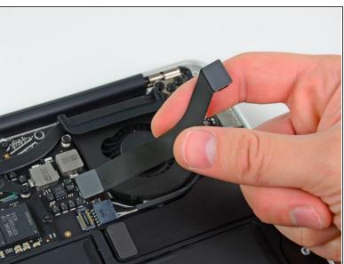
The following connector has an especially deep socket. Use care when disconnecting it.
