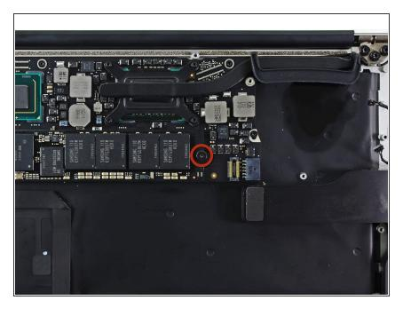
Remove the single 2.85 mm T5 Torx screw securing the SSD to the logic board.
