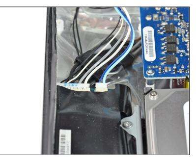
• Disconnect the two inverter cables at the top edge of the inverter using the method explained in the previous step.
