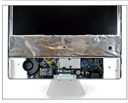
• Tape the EMI shield to the face of the display to keep it out of the way.
