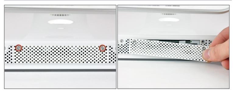
Loosen the two Phillips screws securing the access door to your iMac.
