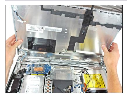
Rotate the display until it is nearly perpendicular to the rear case and lift it up to peel it off the EMI shield stuck to its top edge.
