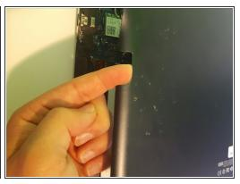
Press the button to release the bottom cover.
