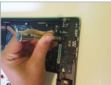
Remove the five 4mm Phillips #00 screws from the motherboard retaining brackets.
