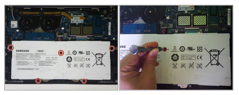
Remove the five 4.3mm Phillips #00 screws from the battery.
