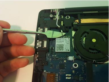
• Disconnect the black and white antenna cables from the Wi-Fi card.
