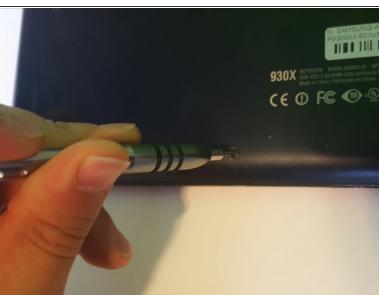
Remove the ten 4.3mm Phillips #00 screws from the bottom cover of the laptop.
