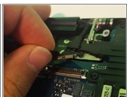
Disconnect the display cable from the motherboard.
