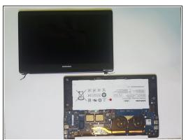
Place the screen on its back side and hold the battery-side of the laptop. In an upward motion, remove the back set off and set it aside.
