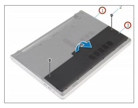
Using a plastic scribe, gently pry the base cover off the computer base.
