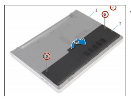
Remove the screws that secure the base cover to the computer base
