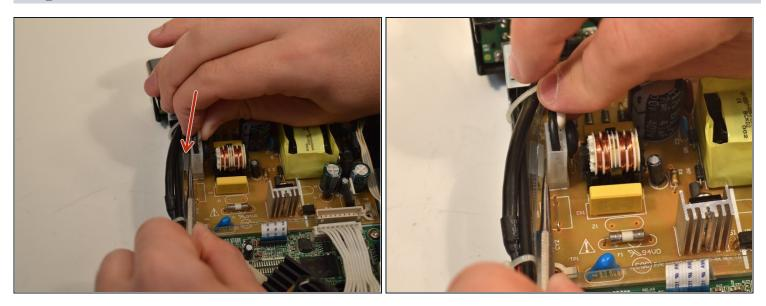
Press down on the plastic flap to unlatch the white clip on the edge of the power supply board.
