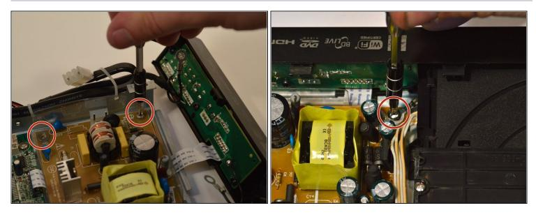
• Remove the 4 screws holding the power board to the body of the device.
