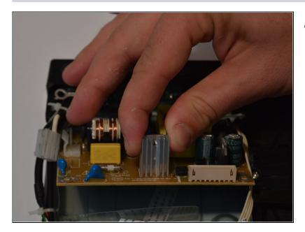
• Remove the power supply board.
