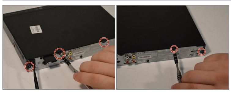
• Remove the four 5mm Phillips #1 screws that connect the black outer shell to the silver back of the device.
