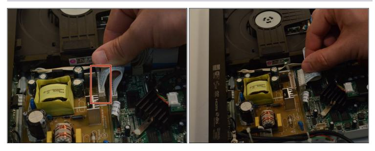
• Remove the 9-pin white wire from the power board (brown) that connects to the motherboard (green).
