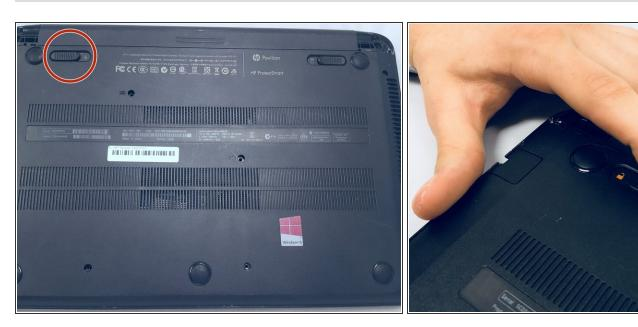
Flip the computer over and move the battery lock switch to the "unlocked" position (marked by an orange lock icon).
