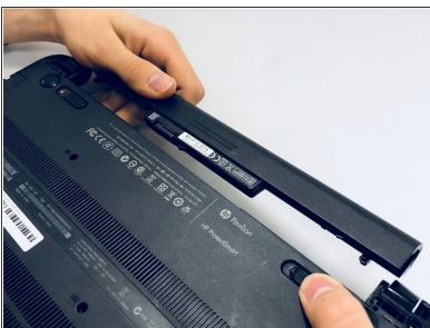
Carefully pull the battery away from the device.
