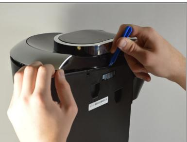
Separate the side panel from the top frame of the brewer, using the blue opening tool for help if necessary.
