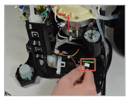
Pull out the white tab that has the wires that connect the Water Sensor to the water pump.
