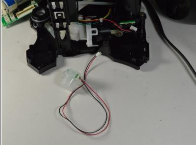
Pry the water sensor out of the frame on the base of the brewer and remove it from the device.
