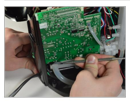
Using the metal spudger, snap the circuit board out of the latches on the bottom of the board.
