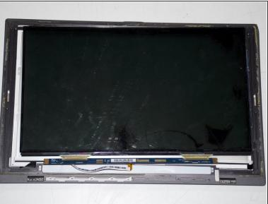
Unscrew the two 2 mmm screws that line the screen control board using a Phillips #1 screwdriver.
