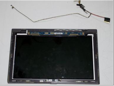
Disconnect the LCD connector from the screen housing by pulling the connector.
