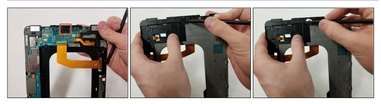
Flip over the device, and carefully push the Rear Camera out of its framing using the spudger.
