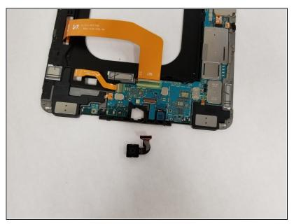
• Remove the Rear Camera from the device.
