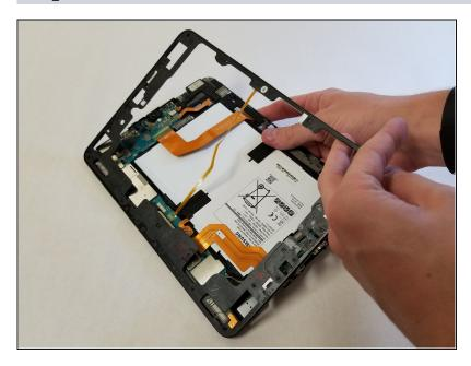
The midframe should snap off from the device's motherboard.
