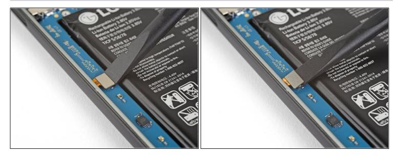
Use the flat end of a spudger to disconnect the left Active Edge sensor connector.
