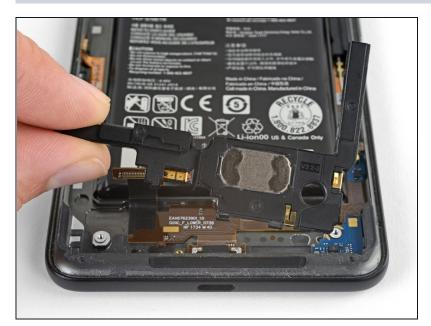
Remove the loudspeaker from the phone. Compare your new replacement part to the original part—you may need to transfer remaining components or remove adhesive backings from the new part before installing.
