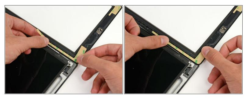
Place the remaining thin L-shaped adhesive strip on the top right corner of the front panel, near the camera mounting bracket.
