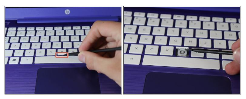
• Using a black nylon spudger, lift the key from the bottom of the key up.
