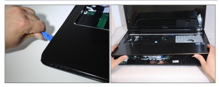
⚠ Do not proceed without holding the laptop screen/lid for support. The screen is very heavy and may cause the device to fall if not held and supported.
