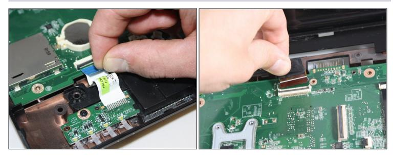
• Flip up the black flaps over the two cables pictured and pull the cables out.
