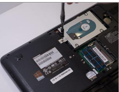
Locate and unscrew the five 3.5mm screws holding the hard drive in place using the J1S Phillips head screwdriver
