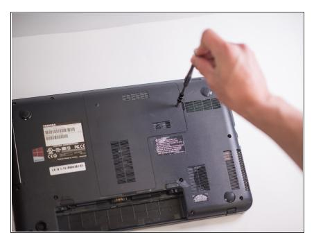
Remove the 7mm Phillips screw located on the back panel of the device using the J1S Phillips head screwdriver.
