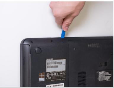
Insert a plastic opening tool and follow the edges to open the panel.
