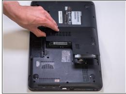
Pry the back panel out of the laptop using the spudger tool
