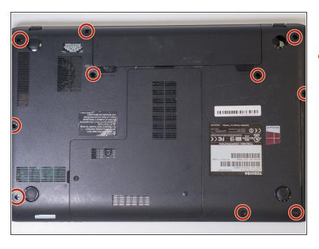
Remove the ten 7mm screws located on the bottom of the laptop using the J1S screwdriver.
