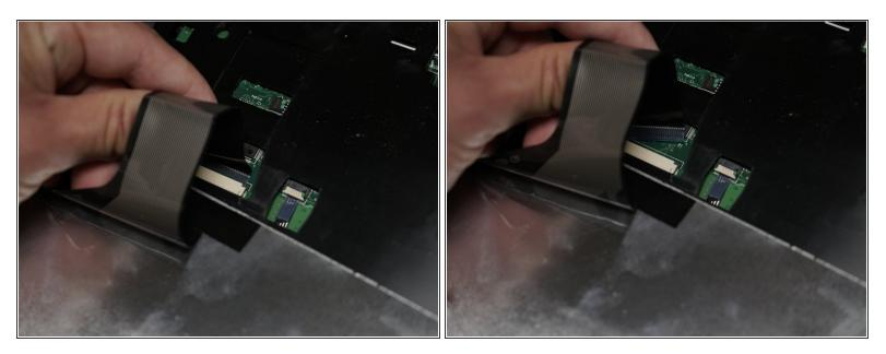
• Pull out the connector attaching the keyboard to the main body of the laptop.
