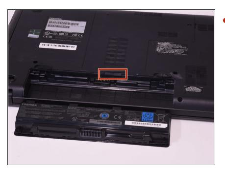
Holding the left tab in place, use the groove located between the two tabs to pry the battery up and out.
