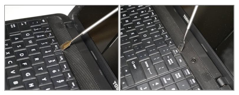
• Carefully separate the keyboard from its assembly by pulling it out with the opening tool.
