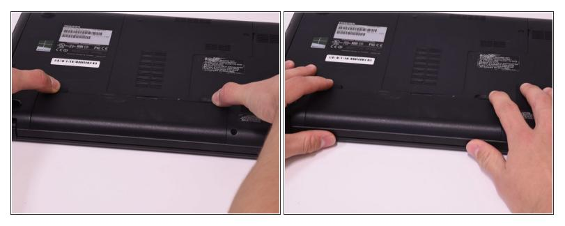
Use two fingers to pull the ridged lock tabs on the bottom of the computer toward the edges. This
