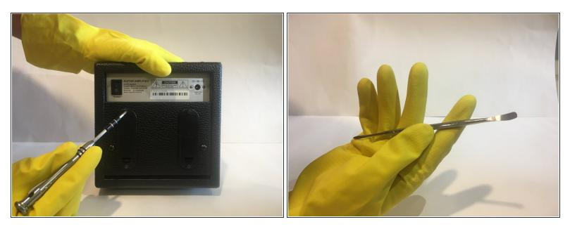
(i) There are several items you will need before starting. You will need: a pair of cleaning gloves, safety glasses, a screwdriver, a metal prying spudger (see picture 2), several Q-tips, distilled vinegar, 2 nine-volt batteries (for replacing damaged batteries), and one small plastic bag.
