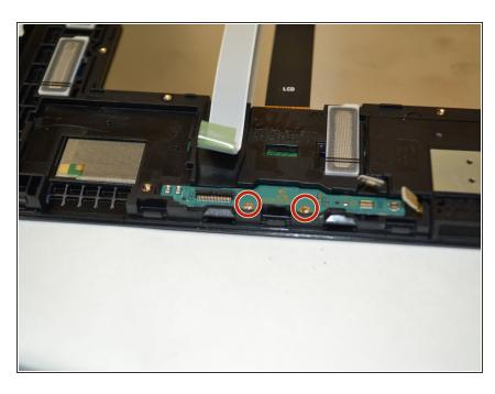
Using your Phillips #000 screwdriver Remove the two 4mm Phillips #000 screws from the home button.
