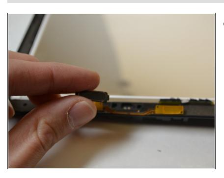
Remove the home button by sliding it to the left or right while pulling up.
