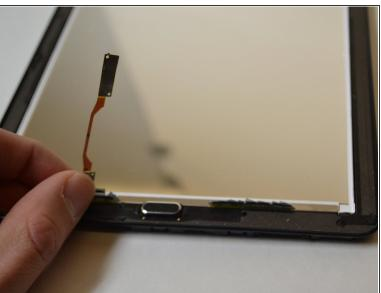
• Locate the Home button on the front of the panel and carefully lift the gold ribbon surrounding it from RIGHT to LEFT.
