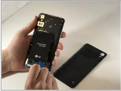
Insert the plastic opening tool into the indent below the battery, and pry up to lift and remove the battery.
