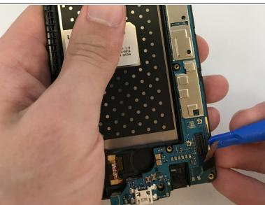
Using a plastic opening tool, lift up display connection until disconnected from the lower right hand of the phone.
