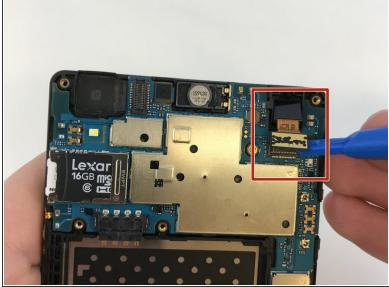
Gently lift the camera ribbon cable until the entire front camera housing is removed.
