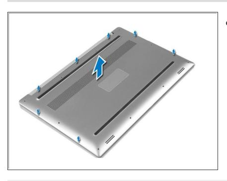
Pry the edges base cover and lift it to remove it from computer.
