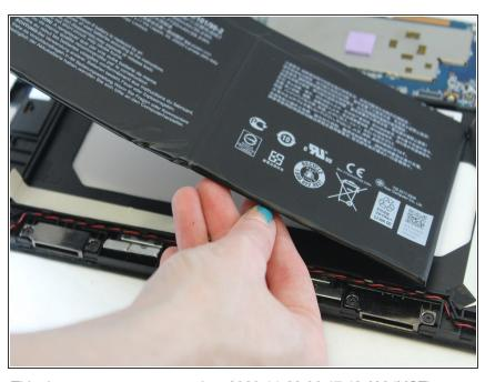
Remove the battery from the device.
