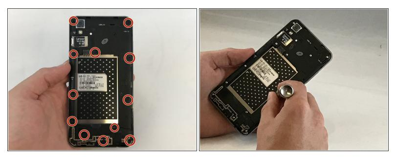
• With a Phillips #000 screwdriver, remove the twelve 3mm screws.
