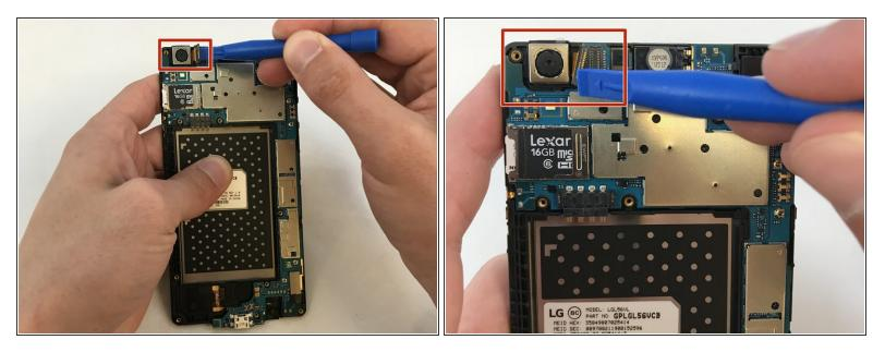
• Gently use the plastic opening tool to pinch off camera connection tab from motherboard.
