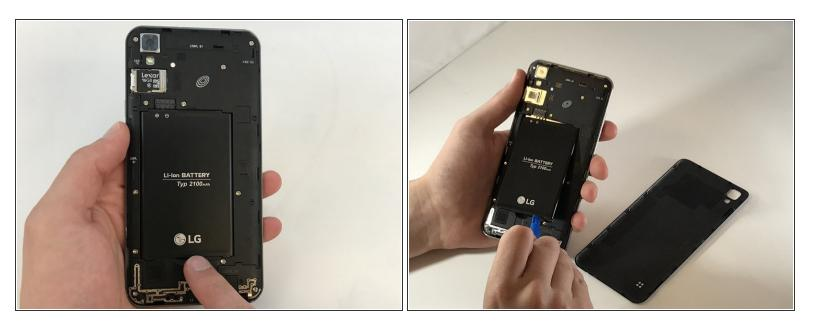
Insert the plastic opening tool into the indent below the battery, and pry up to lift and remove the battery.
