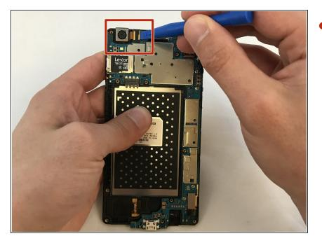
• With the plastic opening tool, gently lift up camera housing and remove.
