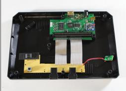
Gently remove the motherboard and the connected tan power switch board from the bottom plate.
