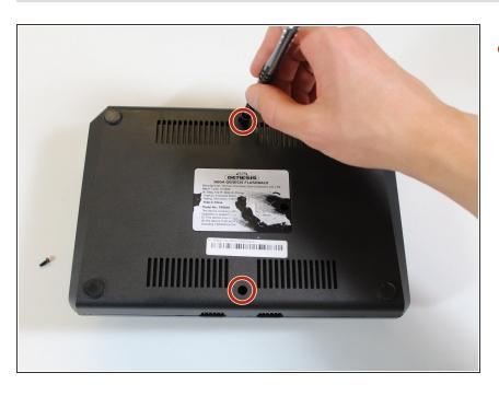
Remove the two visible screws on the bottom with the Phillips #000 screwdriver.
