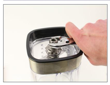
• Using a pair of pliers, pull of the drive shaft coupling.
