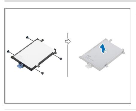
Remove the M3.0x3.0 screws that secure the hard drive. Lift the hard drive from the bracket.
