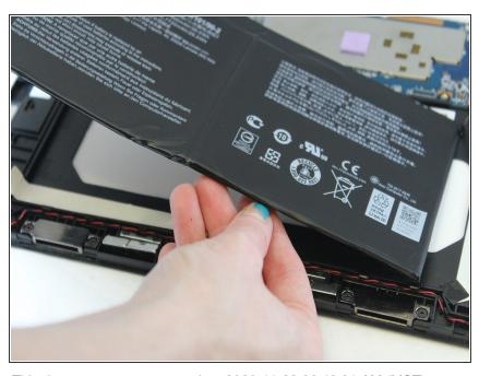
Remove the battery from the device.
