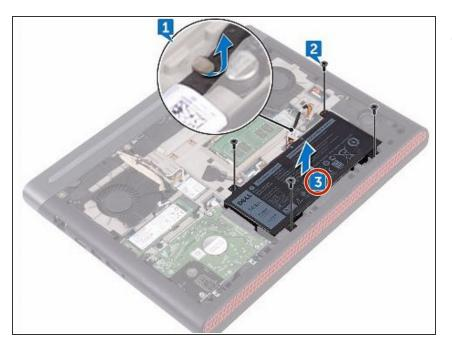
• Lift the battery off the computer base.
