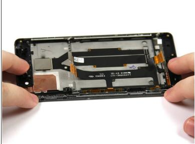
Push down the side of the screen that you just removed screws from.
