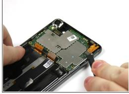
• Use a spudger to pry up the six motherboard connectors.
