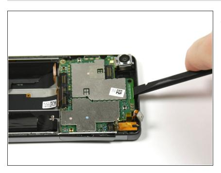
Use the spudger to separate the motherboard from the frame.
