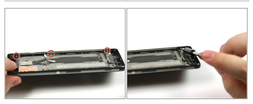
Remove the three 3 mm screws with a Star Bit T5 Screwdriver on the opposite side of the phone.
