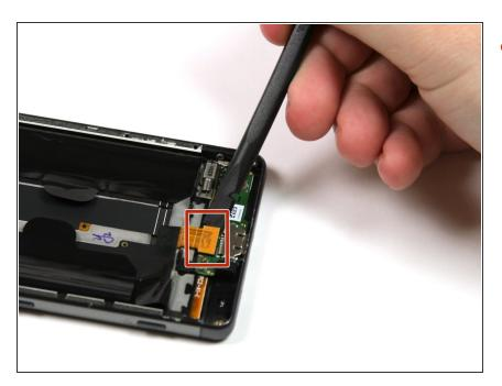
With a spudger, pry up the orange connector that is directly underneath where the loud speaker was just removed.
