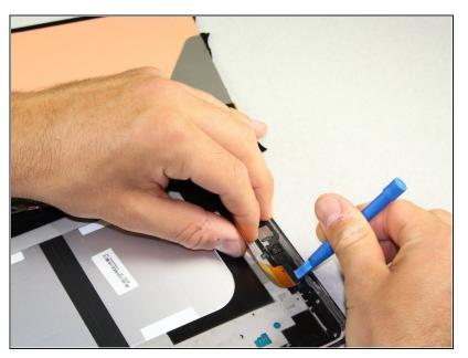
Use the plastic opening tool to get under the connector piece.
