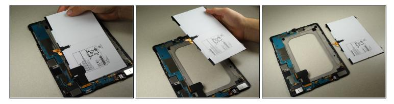
• Gently lift the battery up from one corner using your hands to remove it from the rest of the central panel.
