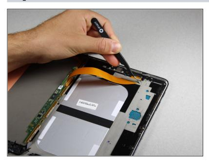
Using the <u>tweezers</u>, gently peel up on the silver tape covering the connector.
