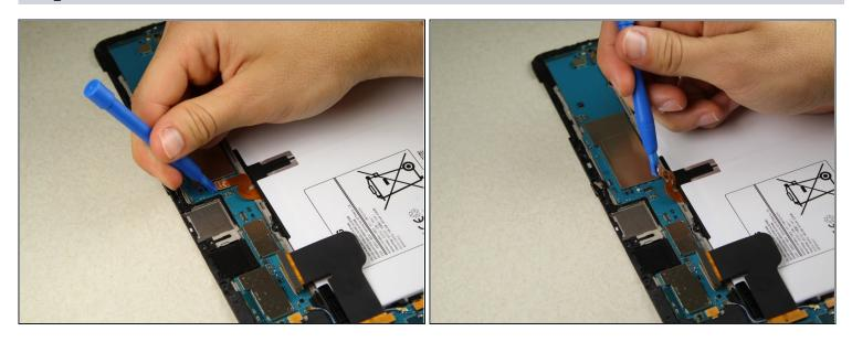
• Gently place the larger plastic opening tool under the cable connector and lift up to detach the connector from the panel.
