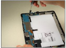
• Remove the 4 black 3.0 mm Phillips head screws from the corners of the battery housing using the screwdriver.
