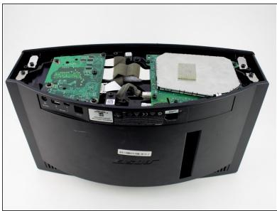
Remove the four 15.5 mm PH2 screws securing the base plate to the device.
