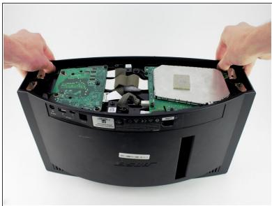
Remove the grille and rear panel by grabbing the corners and pulling upwards and outwards.
