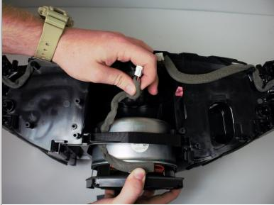
Remove the subwoofer by pulling towards the back of the device while tucking the wire under the plastic enclosure.
