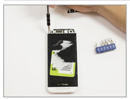
Take out the small 3 mm screw that is on the top left side using a T5 bit.
