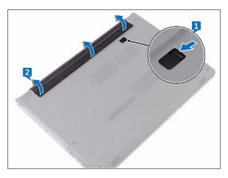
Slide the tabs on the NEW battery into the slots on the battery bay and snap the battery into place.
