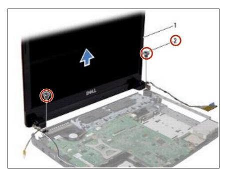
Remove the two screws that secure the display assembly to the computer base.
