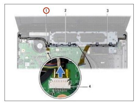
Connect the camera cable to the system board connector.
