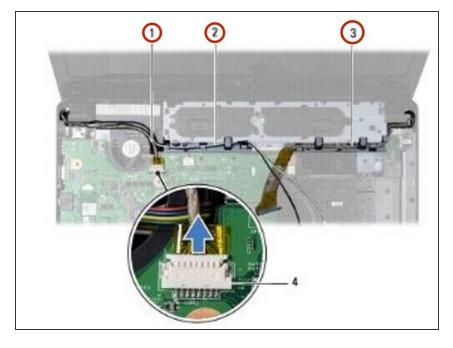
Make note of the Mini-Card antenna cables, camera cable, and the display cable routing and remove the cables from their routing guides.
