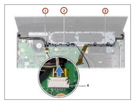
Route the Mini-Card antenna cables, camera cable, and display cable through the routing guides.
