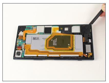
Place the spudger under the top right frame piece and lift to loosen it.
