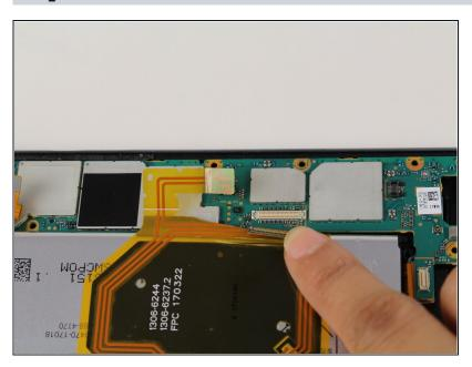
Pull the metal tab of the connector towards you with your fingers to disconnect the pins.
