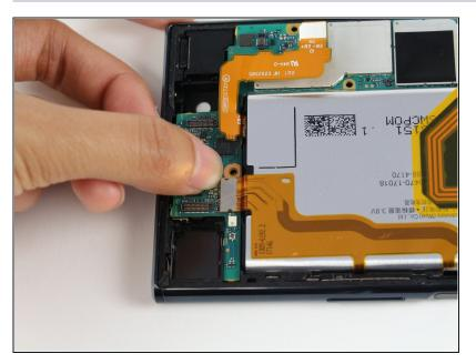
Insert your nail under the metal part of the bottom left connector.
