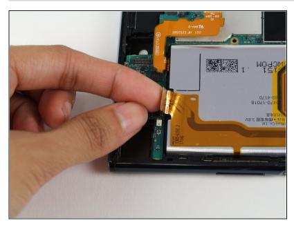
Push the bottom left connector with your finger to disconnect it.
