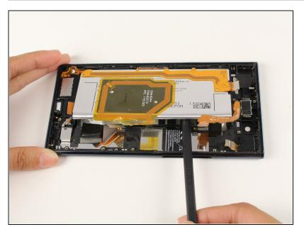
Insert and push the spudger underneath the other sides of the battery to further loosen it.
