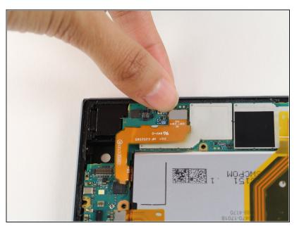
Insert your nail under the top left connector and push to disconnect it.
