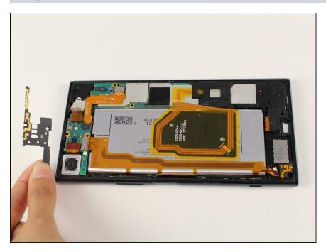
• Grab hold of the bottom left frame and lift out carefully.
