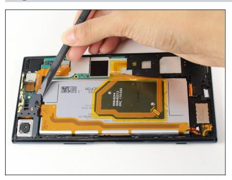
Insert the spudger under the bottom left frame and lift, try to lift vertically to wedge it out.
