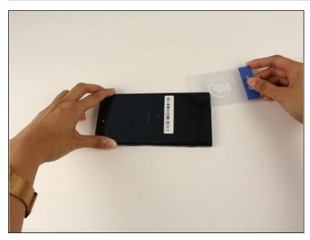
Slide a thin <u>plastic card</u> under the back panel and around the perimeter of the phone to remove the adhesive.
