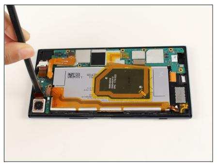
• Insert a spudger under the tab above the camera and lift to disconnect it.
