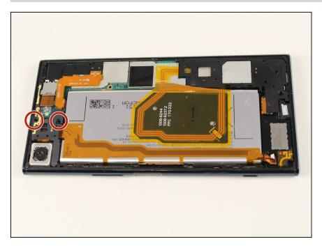
Remove the two bottom left 3.9 mm Phillips #000 screws.
