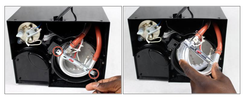
• Remove the two 14mm Phillips head screws that hold the heating coil in place.
