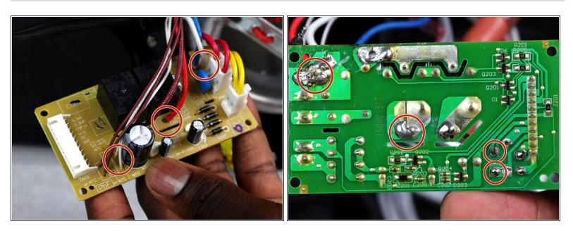
• De-solder each of the four wires connecting the coil to the circuit board.
