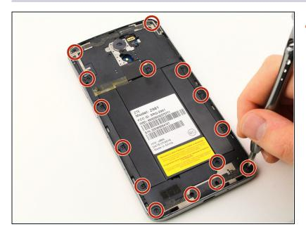
• Using the Phillips #00 screwdriver, remove the 15, 3.0 mm rear panel screws located around the perimeter of the phone.
