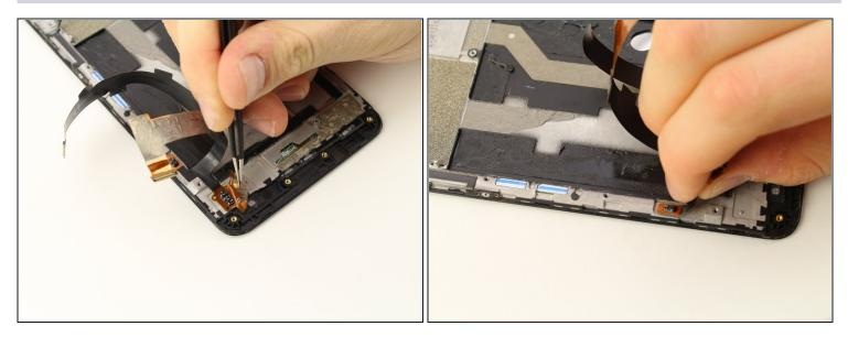
• Peel the flex cables off where they are attached to the frame.
