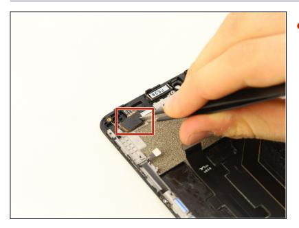
Disconnect the digital flex cable connector, located at the top left of the phone, using a pair of <u>tweezers</u>.
