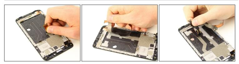
• Using your fingers peel up the LCD flex cables. These cables are black and flat.
