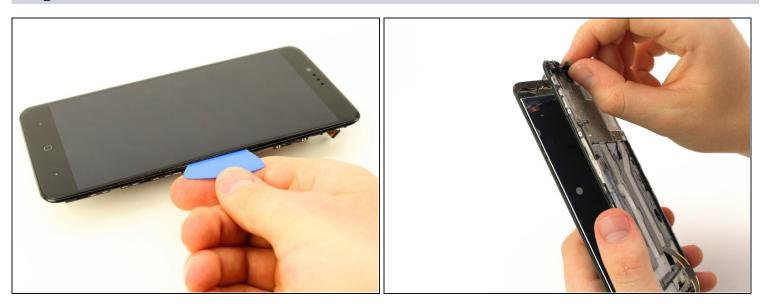
• Insert a plastic opening tool between the screen and the rear case and separate it carefully, starting at the bottom.
