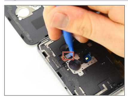
Remove the fingerprint sensor flex cable, using the plastic opening tool to lift it out.
