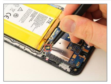
Use tweezers to remove the antenna. The antenna comes up on the right side of the phone, by the battery, and is attached to the motherboard.
