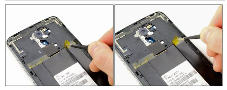
• Using the tweezers, peel back the yellow Kapton tape located on the right side of the phone.
