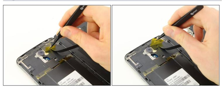
• Remove the yellow Kapton tape by using the <u>tweezers</u> to peel it up and away from the device.
