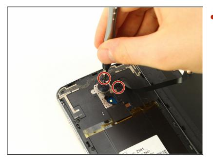
Using the Phillips #00 screwdriver, remove the two 3.0 mm screws located near the top of the phone, next to the rear camera.
