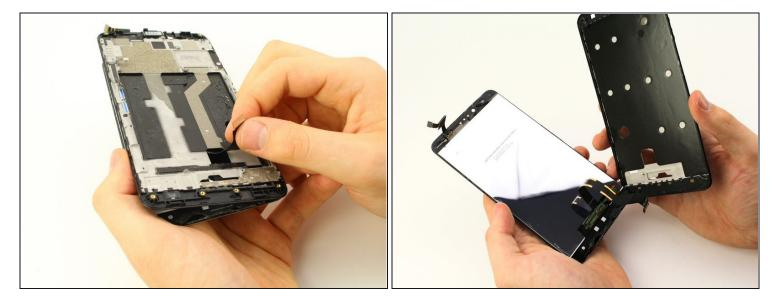
• Push the digitizer flex cable through the hole in the frame to separate the LCD from the phone.
