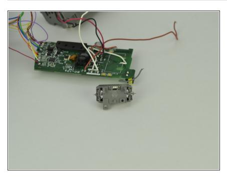
The flash bulb should now be detached completely from the circuit board. To reassemble your device, follow these instructions in reverse order.
