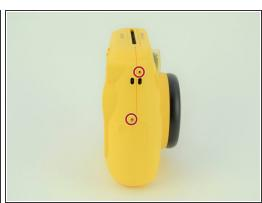
Remove the six 4.5 mm #00 Phillips screws from the bottom, left, and right sides.
