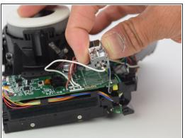
Remove the flash bulb from the circuit board by shifting it towards the side with the motor and lifting.
