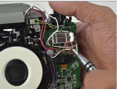
Once the shell is off, remove the one 6.5 mm screw that is attached to the flash bulb using a Phillips #00 screwdriver.
