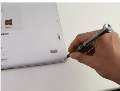
Remove the eight 3 mm screws using the Torx T5 driver by inserting the screwdriver into each screw and rotating counterclockwise.
