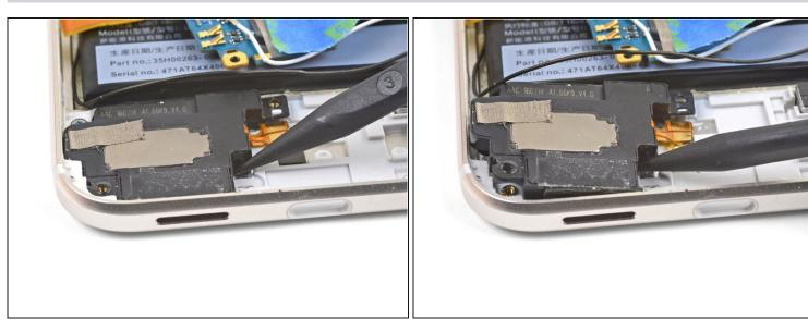
• Use the point of a spudger to pry up and loosen the loudspeaker from its recess.
