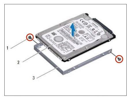
Replace the two screws that secure the hard-drive bracket to the hard drive.
