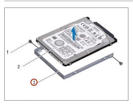
To avoid damage to the hard drive, gently slide the hard-drive bracket away from the hard-drive slot.
