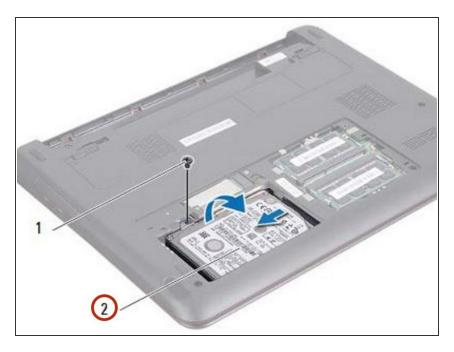
Place the **NEW** hard-drive assembly in the computer base.
