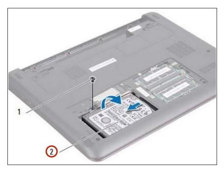
Slide the hard-drive assembly into the connector on the system board.
