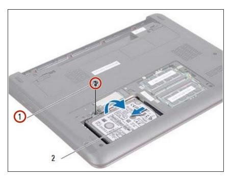
Replace the screw that secures the hard-drive assembly to the computer base.
